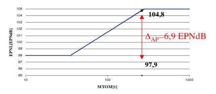
Chapter 3 limits for the three measurement points of Flyover (FO), Sideline (SL) and Approach (AP) noise can be calculated from the formulas contained in ICAO Annex 16 Volume I.
