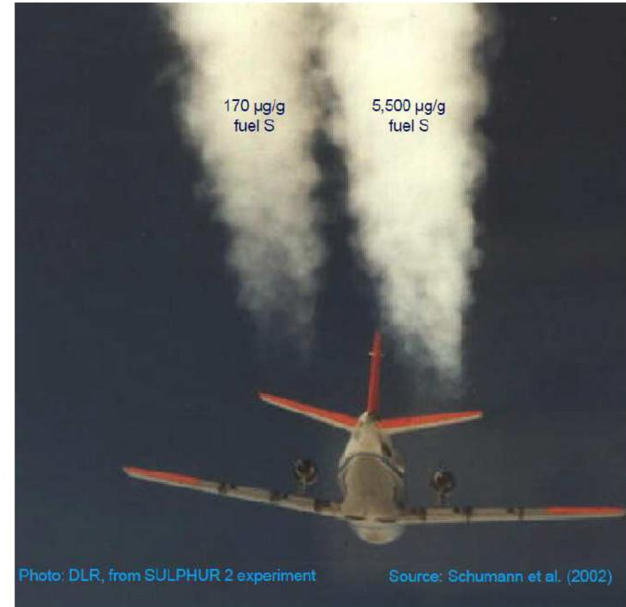
Figure 4-2 Effect of FSC on contrail formation (reproduced with kind permission of DLR)
